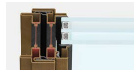
Section - Frame + Sash total is 47 mm
