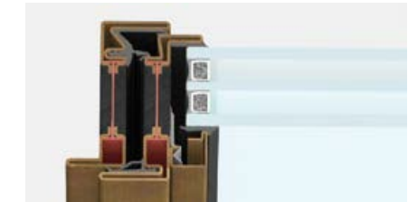
Section - Frame + Sash total is 47 mm
