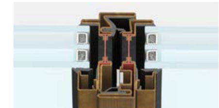
Middle Section - Frame + Sash total is 62 mm
