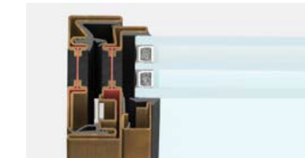
Section - Frame + Sash total is 47 mm
