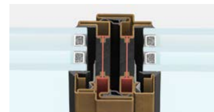
Middle Section - Frame + Sash total is 62 mm
