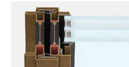
Section - Frame + Sash total is 47 mm
