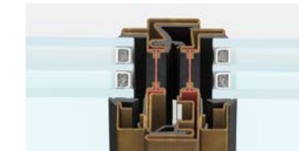
Middle Section - Frame + Sash total is 62 mm
