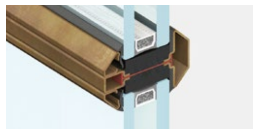
glazing bar | frame section 36 mm
