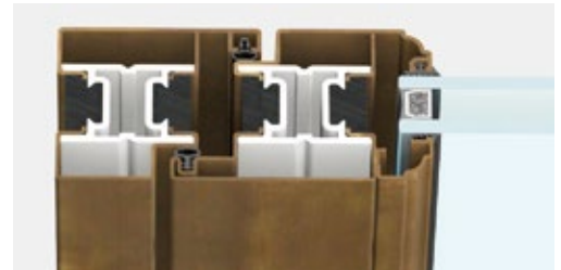
lateral section | frame section 132 mm
