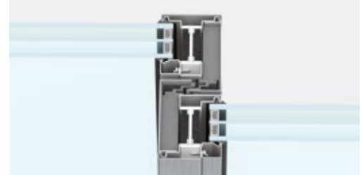
reduced central section | frame section 69mm
