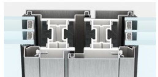
central section | frame section 156 mm
