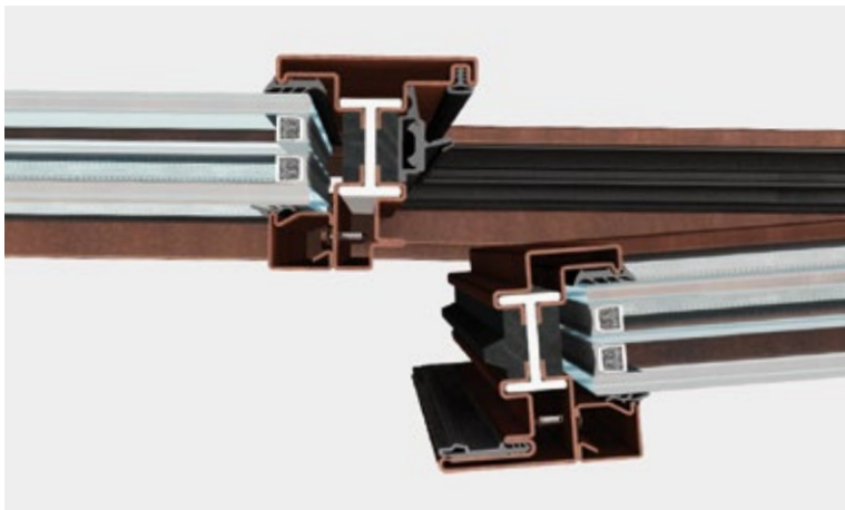
double-sash window central section | frame section 110 mm
