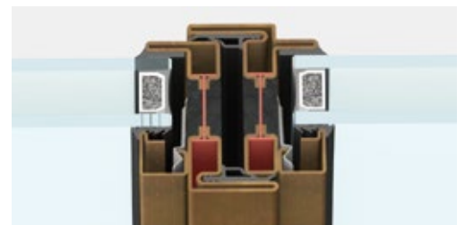
central section | frame section 62 mm
