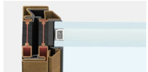
lateral section | frame section 47 mm
