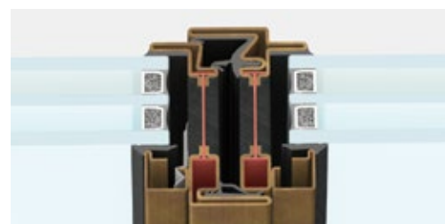
central section | frame section 62 mm
