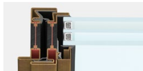
lateral section | frame section 47 mm
